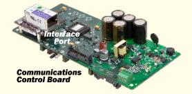
**Efficient Modularity -** The Breaker Interface Modules (BIM's) use circuit boards in a three breaker modular configuration. This allows the user to purchase only the number of controlled circuit breakers needed. As demand rises, the BIM's are field-upgradable to increase the number of controlled circuit breakers.
